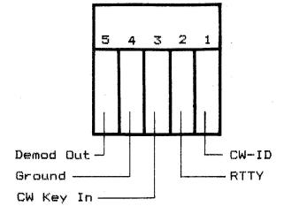
Strip the outer insulated shielded end of the cable, but do not strip the colored wires. Place the connector face up, with the open side up, and press the unstripped wires directly onto the pins in each of the five chambers. (See Diagram) Do not push the wires in from the end, but rather directly down onto the pins.
