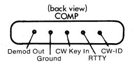
These five lines are used to receive information from The Interface and to control it. The functions of the lines are as follows.
