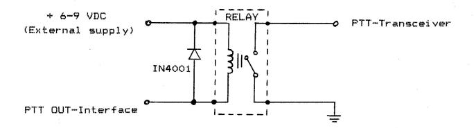
We suggest you use a Radio Shack 6-9 volt DC miniature relay (part number 275-003) or equilivent. DO NOT use internal power from The Interface for the relay. Use power from an adapter or external power supply.
